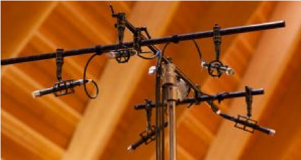
Figure 1 – Surround microphone configuration based on Decca Tree
