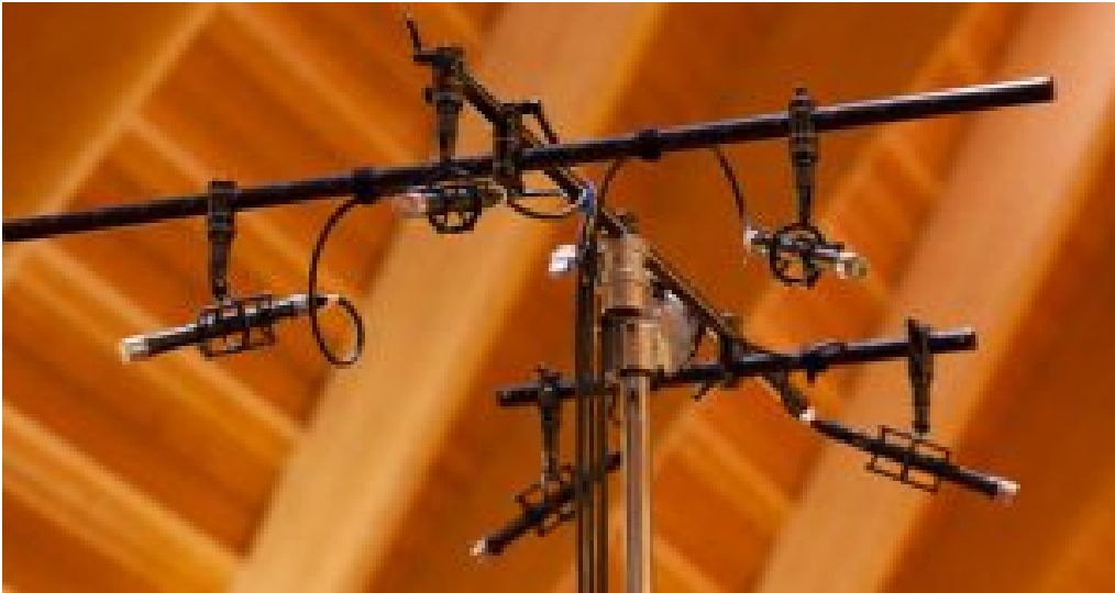
Figure 1 – Surround microphone configuration based on Decca Tree
