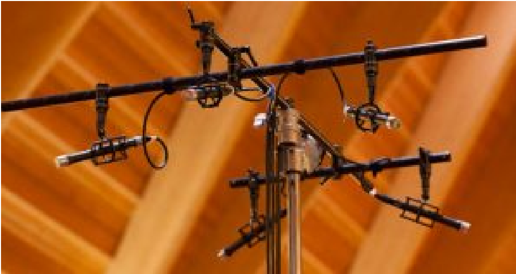
Figure 1 – Surround microphone configuration based on Decca Tree
